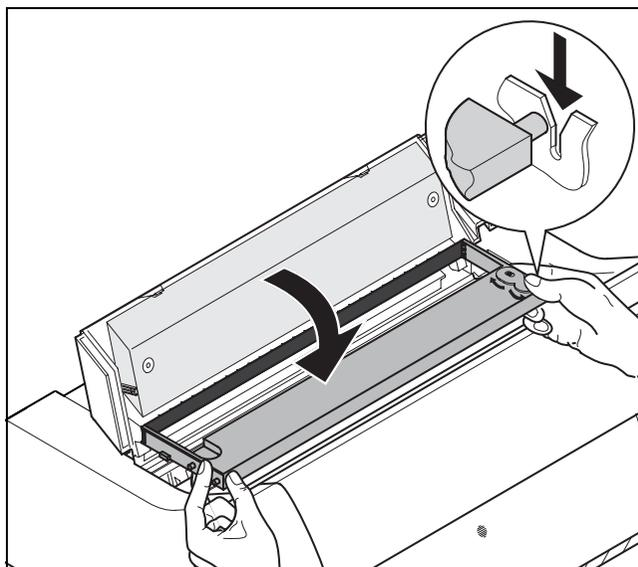
Slightly tilt the ribbon cassette forwards and thread in the ribbon between the coloured insertion tongue and the ribbon support (transparent plastic plate).
