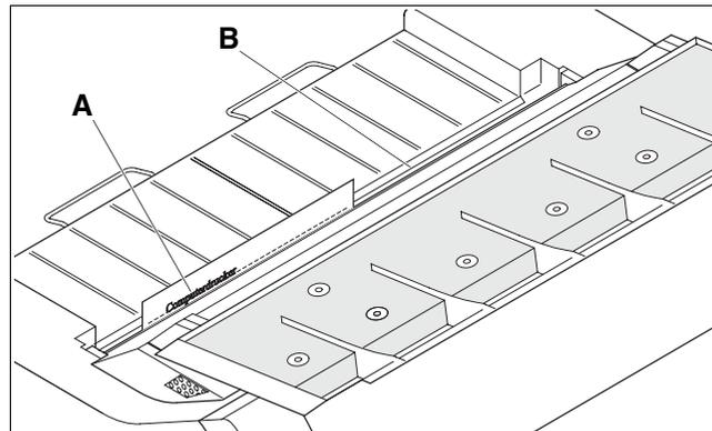
The paper is fed to the position where the bottom edge of the first printing line **A** is aligned with the tear edge of the top cover **B**. The factory setting for the first printing position (TOF) is 12/72".
