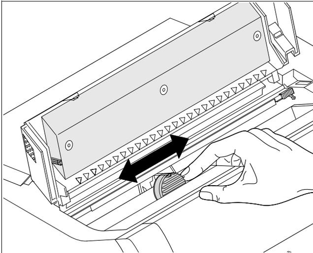
Move the print head carriage backwards and forwards several times. If the ribbon is correctly seated, there must be no perceptible resistance.
