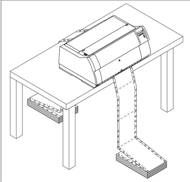
If you expect that frequent forward and reverse feeds will occur, you should place the printer as shown in the figure, if possible.
