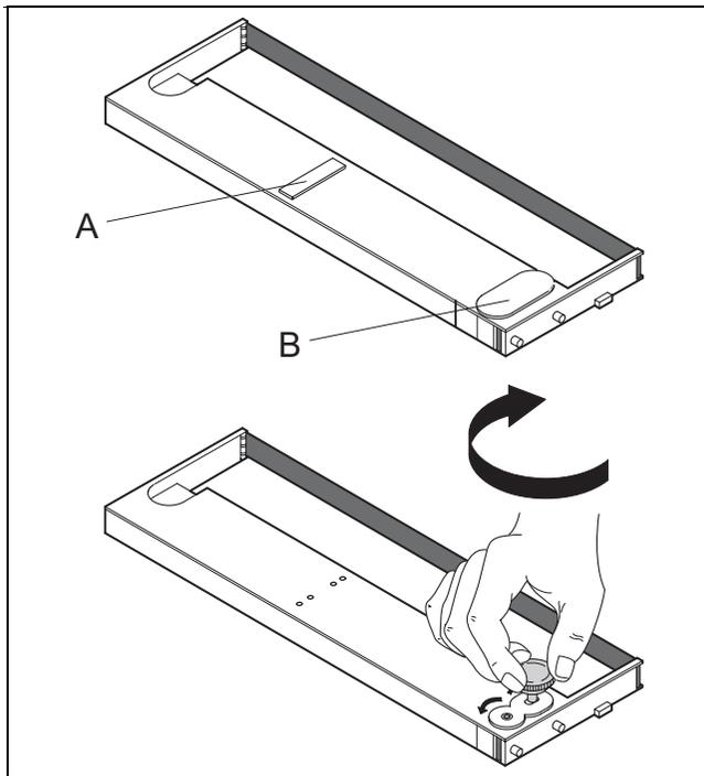
Remove the coloured protections **A** and **B**.
