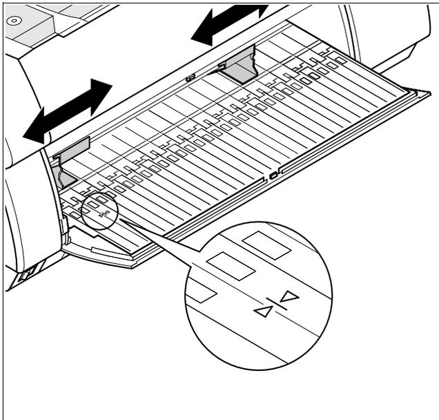
Align the left paper guide with the mark on the left of the single sheet input tray. Adjust the right paper guide to the width of the paper used.
