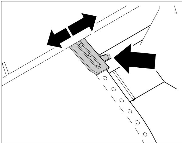
Open the coloured latch lever of the right-hand tractor and align it to the paper width.
