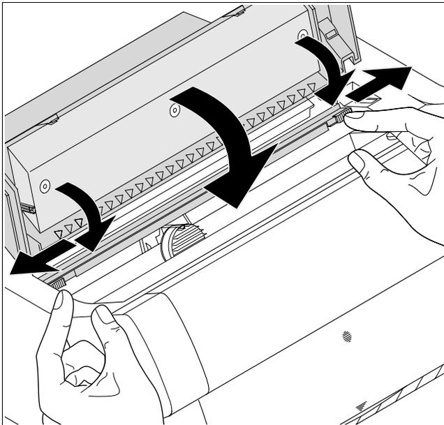
Press the friction mechanism down until it clicks into place. Close the front section of the top cover.
