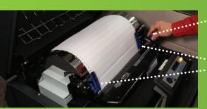
THE NEW MICRO PLATEN ADJUSTER = Improved print reliability and handling for a wider variety of forms, such as multi-part, heavy, recycled and light stock.
