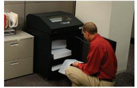
FRONT PAPER ACCESS = Load forms and retrieve printed output from the front of the 6600Q cabinet. This option allows you to better utilize office space by placing the printer against a wall.
