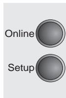
Make sure that the printer is in offline mode; press the **Online** key, if necessary.
