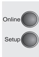
Press the **Online** key to set the printer to ready status. When the printer receives data from the computer, the single sheet is automatically loaded. Press the **Load** (4) key to load the single sheet before starting the printout.
