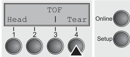
Press the **Tear (4)** key. The printer performs a form feed.
