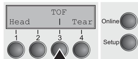
Press the **TOF** (3) key. The printer performs a form feed.
