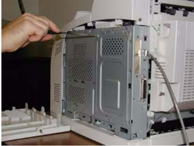
5. Once the thumbscrews have been removed, pull the side panel away from the printer by the top edge as show below.
