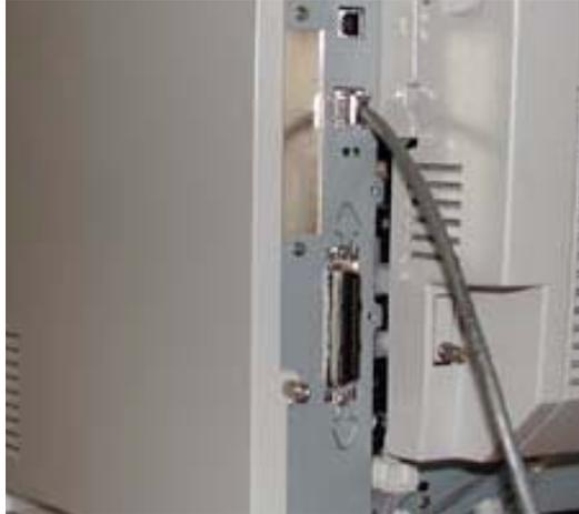
4. Turn thumbscrews on controller assembly counterclockwise until loose and gently pull cover towards you to remove from printer.
