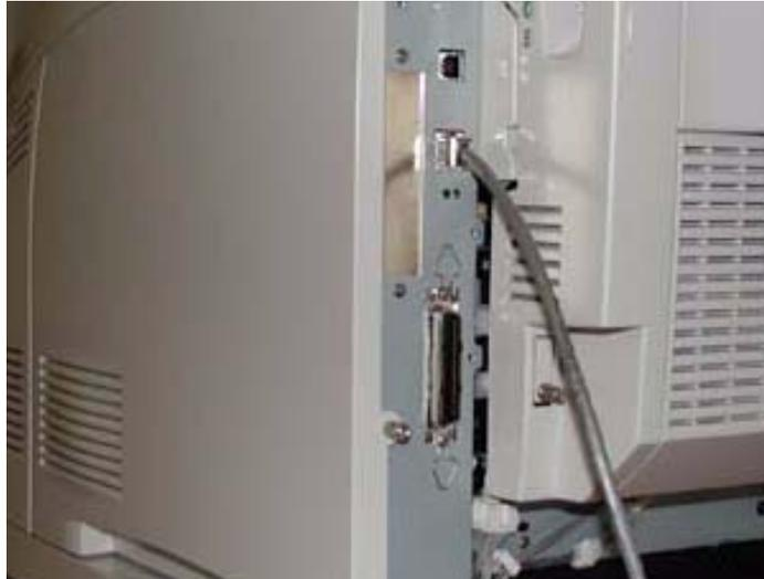
4. Turn thumbscrews on controller assembly counterclockwise until loose and gently pull cover towards you to remove from printer.
