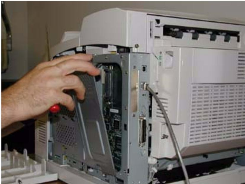
6. Locate the area of the controller identified as “Hard Disk”. Align the hard disk within the designated area and gently move up to ensure the 44-pin male connector of the hard disk is connected to the 44-pin female connector on the controller assembly
