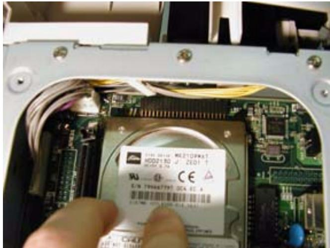
8. If there is improper alignment, remove the Hard Drive and reinstall.
