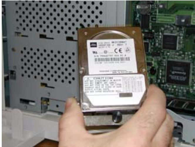
7. Be sure to align the Hard Drive as depicted by the alignment drawing on the controller, making sure that the two top pins to the left of the connector are free standing and not connected.
