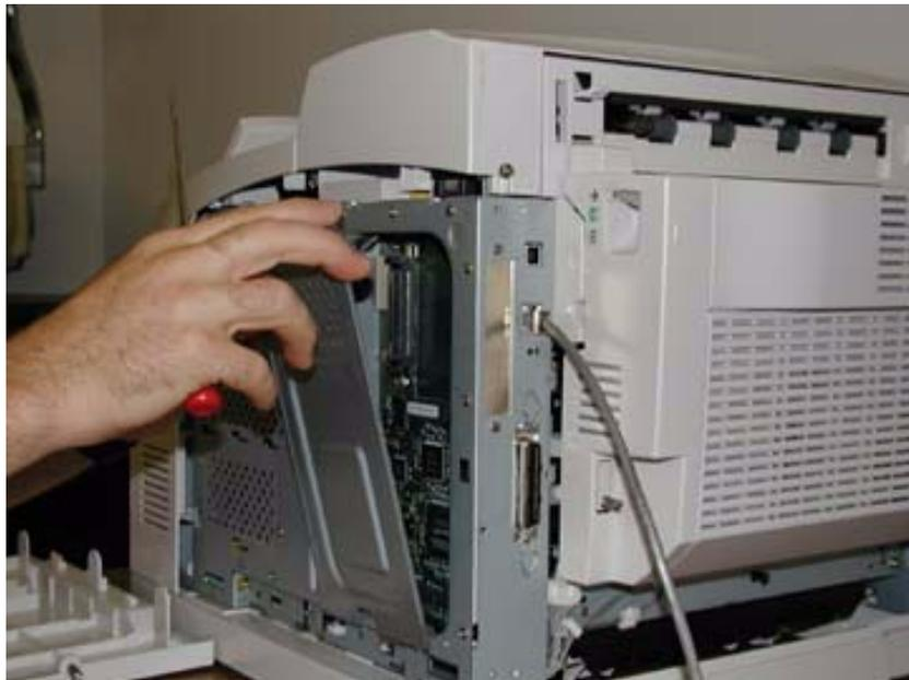
6. Carefully insert a DRAM DIMM which is compatible with your printer into DRAM DIMM slot as shown below. When properly seated, gently push down on the DIMM until the side braces close onto
