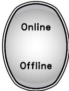
This key toggles the printer between Online and Offline states, or exits from the menu directly to an Online state. When the printer is Online, the indicator will light, and the printer is ready to accept data from the host. When it's Offline, it cannot accept host data. In the Offline state, you may change parameter selections, load paper, and so on.
