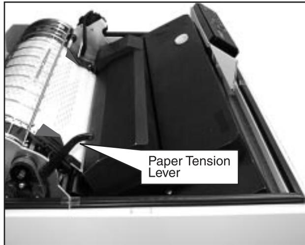
Figure 1–11. Paper Tension Lever
