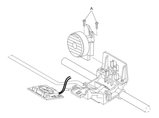
5.2.2 Installing the Printhead
