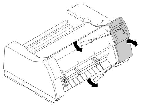
Use a screwdriver to unlock the casing aperture as shown in the illustration and remove it.
