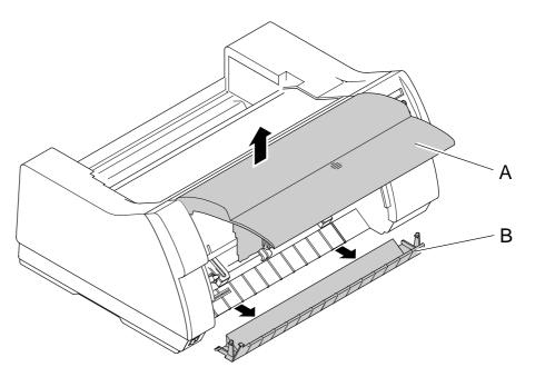
Use a screwdriver to unlock the casing aperture as shown in the illustration and remove it.
